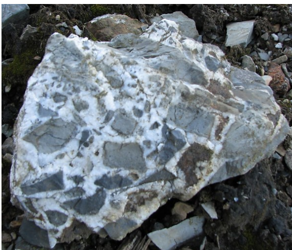
Figure 605: (left) Explosively produced fault breccia, cemented with quartz. Castell mine. (right) Fault breccia containing quartz with galena and pyrite, now weathered to rusty iron oxide. Bwlch Glas mine.
