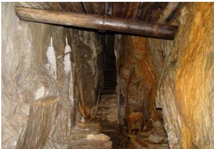
Figure 612: (above left) Stope within the Llewernog mine. (right) Quartz vein containing galena.
