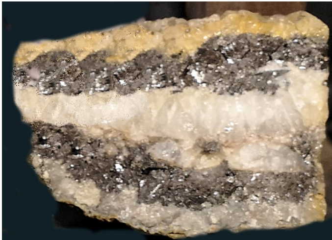
Figure 620: Second phase minerals deposited at Cwmystwyth mine: (left) Quartz and galena vein. Courtesy of Ceredigion Museum, Aberystwyth. (right) Sphalerite.
